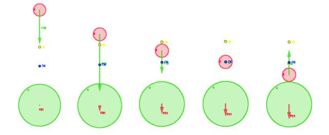
When the two bodies come closer, the force exerted on M2 increases (Newton); but there is a distance (yellow point on the image) from which the force exerted on M2 begins to decrease.
